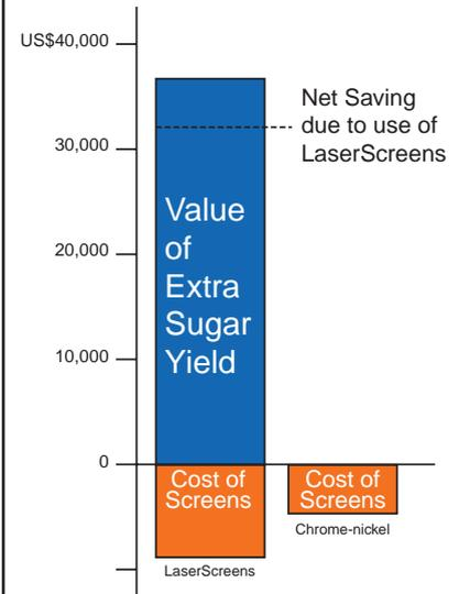
Example Basis: 9,600 tpd (cane) capacity; 0.75 of a unit final molasses purity reduction due to LaserScreens; US\$220 / tonne sugar price.
